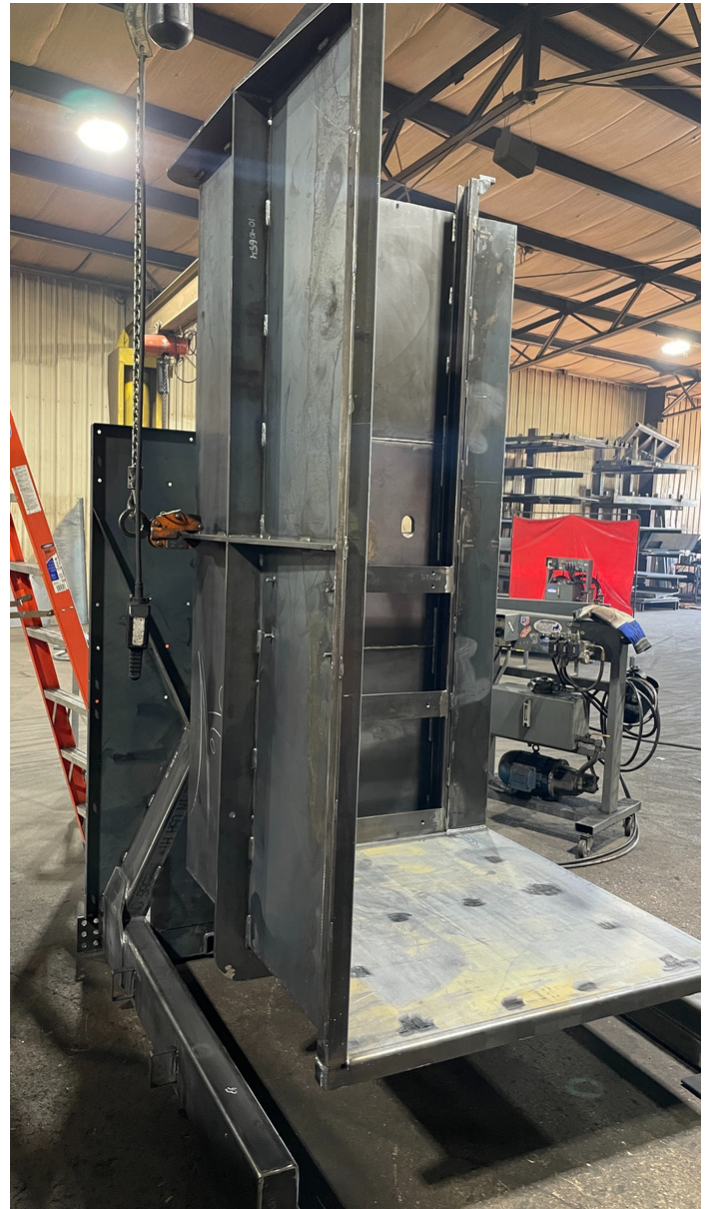
The working shell of a Pallet Inverter for Cherry's Industrial Equipment. A pallet inverter is a piece of equipment that can take loads, sometimes up to 8,000 lbs., and rotate them 180 degrees in seconds.
