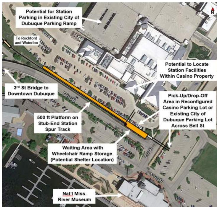
Figure 5: Dubuque Station – 3<sup>rd</sup> Street Spur alternative conceptual layout
